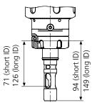
SensoGate® WA 131 M Process adaptation for dairy pipe, DIN 11851 DN 50 ... DN 100, short and long immersion depth (ID)
