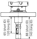
SensoGate® WA 131 M Process adaption for 25 mm Ingold socket, short and long immersion depth (ID)
