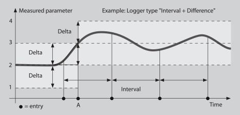
Combined time- and difference-controlled logger: provides high resolution when the measured value changes, saves data volume when the value is constant
